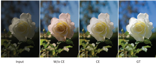
Fig. 4. Visualization of color embedding. Without color embedding, the white semantic objects take significant color shift. W/o CE: without color embedding; CE: with color embedding; GT: ground truth.
