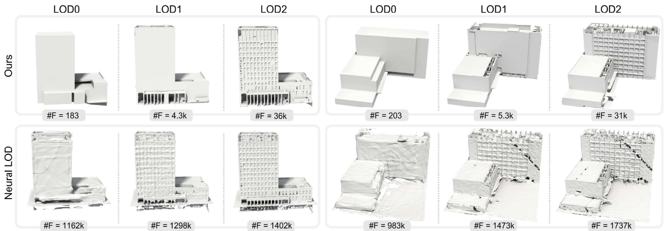
Fig. 12. Comparisons with NeuralLOD. The face number of NeuralLOD-based results are huge even in models with LOD0 layer. Co-LOD effectively reduces the face number while maintaining accurate geometric structures in different LOD layers.
