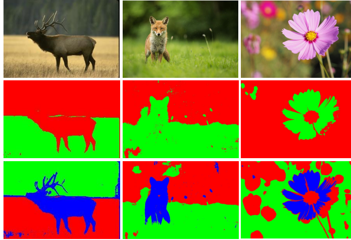
Fig. 6. An instance of GMM-based image segmentation. First row: input images; second row: segmentation results with two classes; third row: segmentation result with three classes.
