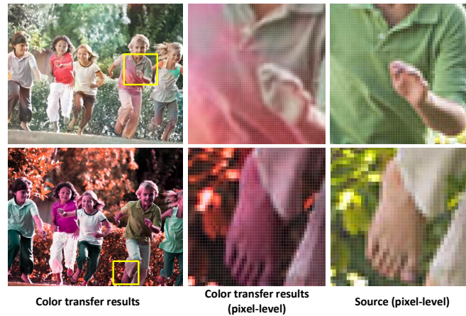
Fig. 14. Two failed instances of color transfer. First row: color transfer result by He2018 [34], the continuity of the color distribution is broken; second row: color transfer result by Lee2020[50], the color deviation is produced which breaks the naturalness of the image.
