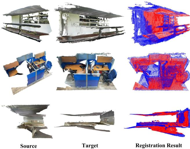
Fig. 1. Instances of KSS-ICP registration results. Point cloud models are scanned by iphone12pro in Nanyang Technological University. In third column, the red point clouds represent the source point clouds; the blue point clouds are target ones. Registration results show that our method can align raw point clouds from source to target.
