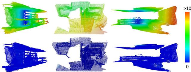
Fig. 2. Color maps of corresponding errors (point distance) between source point clouds and target ones (red to blue: high to low). First row: before registration; second row: after registration. It is clear that the corresponding errors approach zero after our registration.
