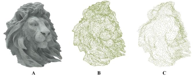
Fig. 6. An instance of simplified point clouds. A: real 3D object; B: scanning point cloud; C: simplified point cloud (2,000 points).
