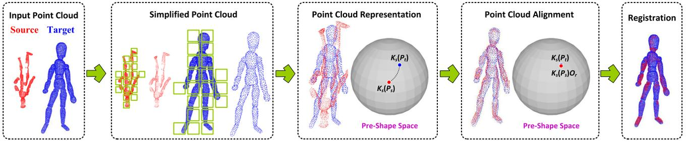
Fig. 3. The pipeline of KSS-ICP. In pre-shape space, the influence of rotation is not removed. Therefore, representations of source and target point clouds in the space have different positions. Our registration is to remove the influence which can be regarded as a practical simulation of KSS mapping. When the two point clouds can be aligned into a same location in pre-shape space, it means that they can be mapped into a same reflection in KSS.
