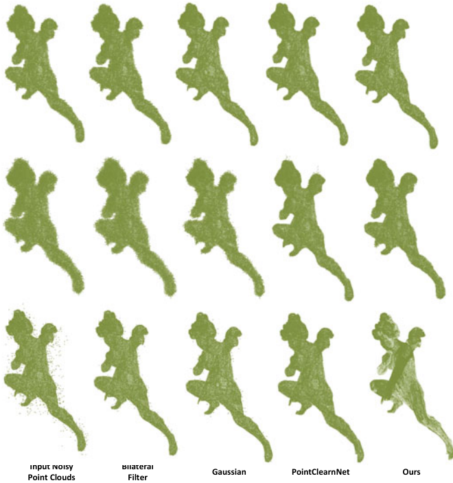
Fig. 12. Comparisons of denoising results. From top to bottom: 0.33 Gaussian noisy models and related denoising results; 0.66 Gaussian noisy models and related denoising results; random outliers and related denoising results.
