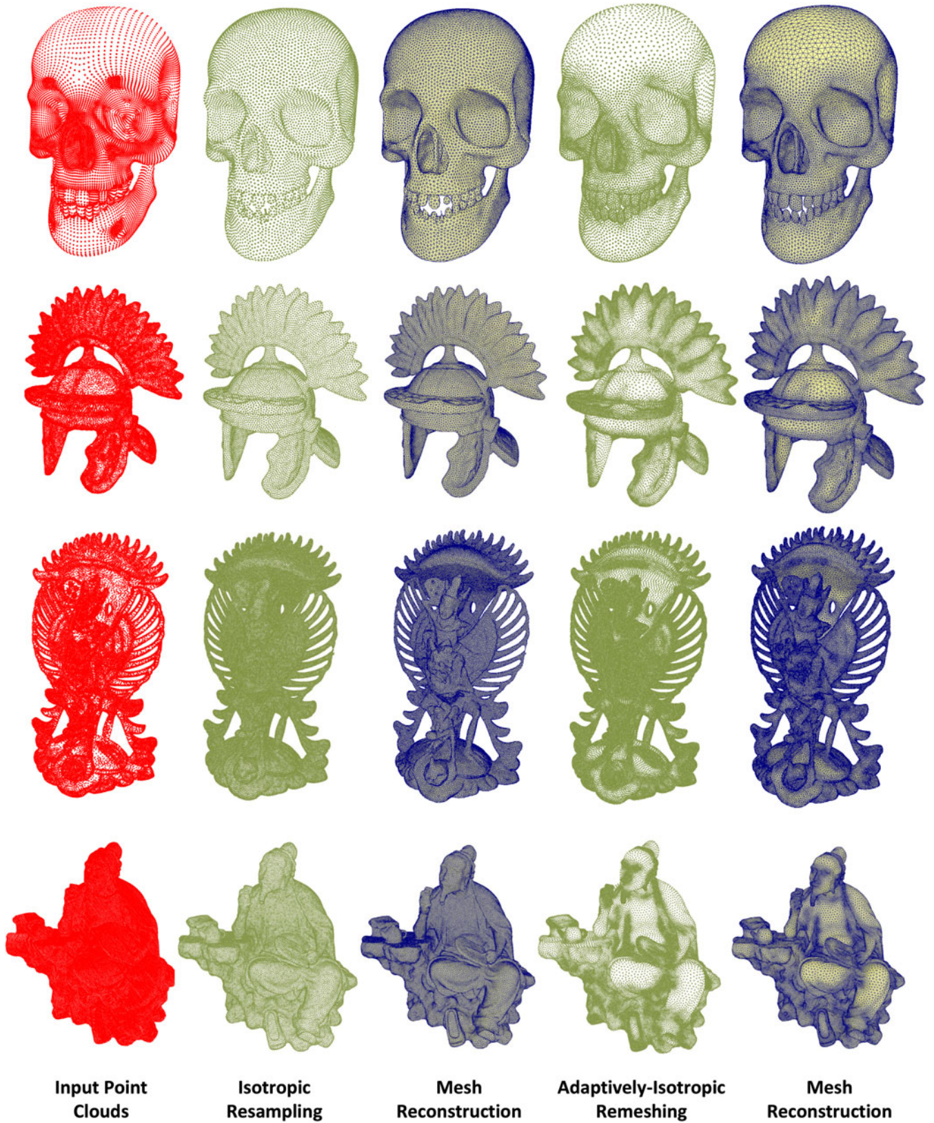
Fig. 21. Some resampling and mesh reconstruction instances by our method. The third column: the mesh reconstruction is based on isotropic resampling; the fifth column: the mesh reconstruction is based on adaptively-isotropic resampling.
