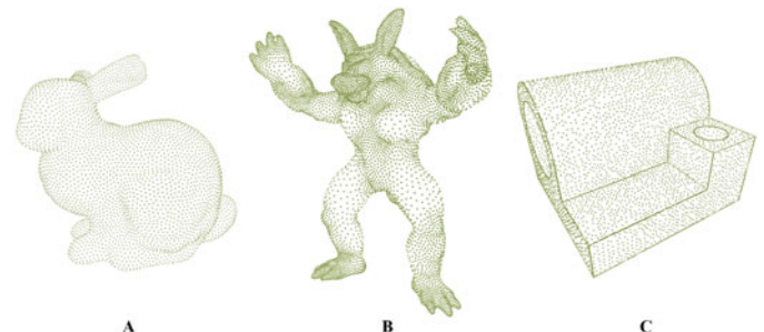
Fig. 11. Some instances of isotropic and adaptively-isotropic resampling results. A: isotropic resampling; B: adaptively-isotropic resampling for curvature sensitive resampling; C: adaptively-isotropic resampling for sharp edge keeping.
