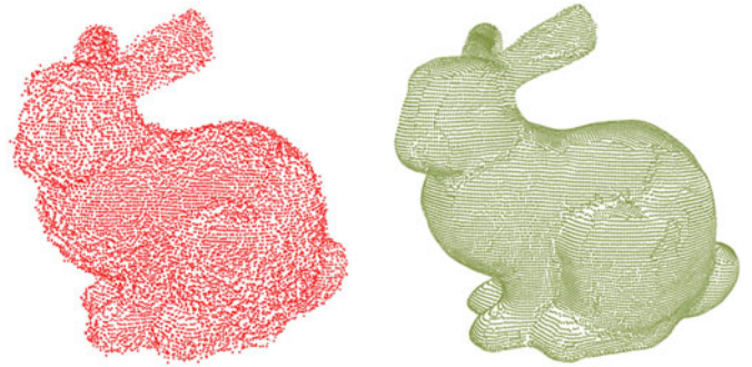
Fig. 3. An instance of denoising result. The red point cloud is the input point cloud with noise; the green point cloud is the denoising result.
